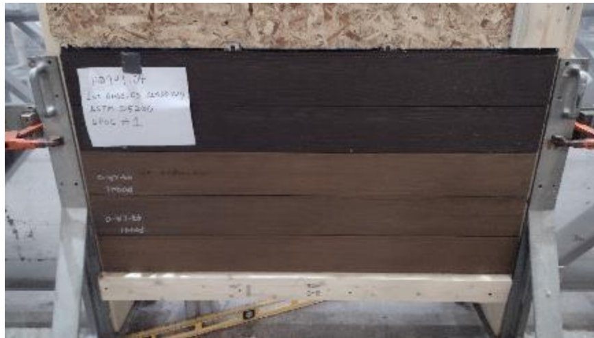
Photo No. 1 Test Specimen #1 Los Angeles Collection, Cladding
